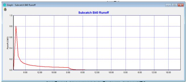
**Figure 4.** The peak flood discharge diagram in the hydrological unit 40 obtained from the SWMM software 4-1 - Evaluation of the transfer capacity of conduits
